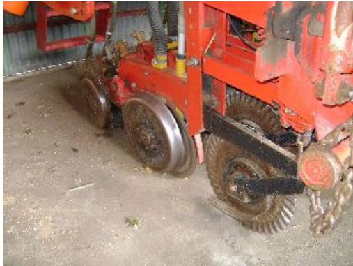
Planting line of the Bertini no-till seed drill
