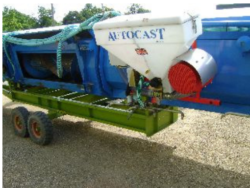
◀ Autocast oil seed rape seed broadcaster mounted on the rear of the Shelbourne Reynolds stripper header
