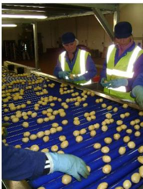
**Grading washed potatoes. The line is capable of processing sixteen 10 kg cases per minute.**
